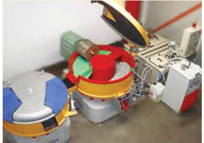
Vibratory machine with magnetic drum separation, waste water treatment system and round vibratory dryer
