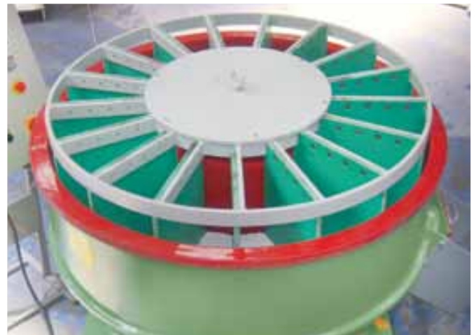
Carousel Vibrator: Round vibratory machine with paddle wheel divider
