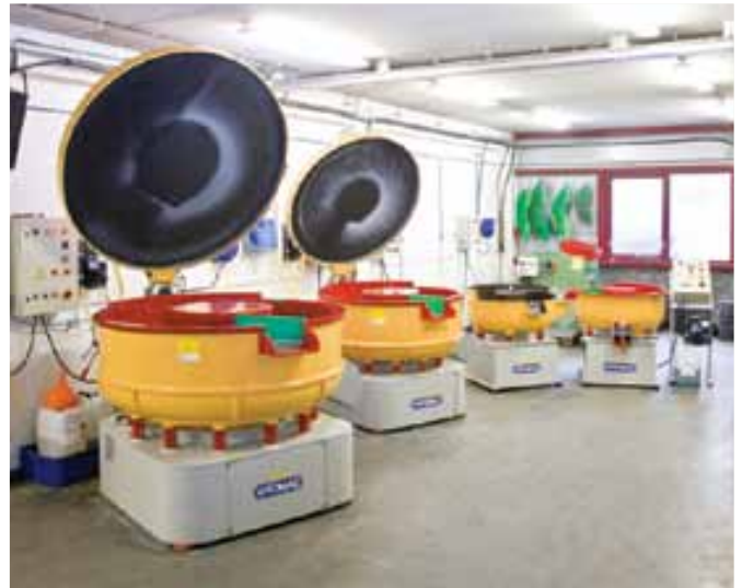
Vibratory machine with magnetic drum separation, waste water treatment system and round vibratory dryer
