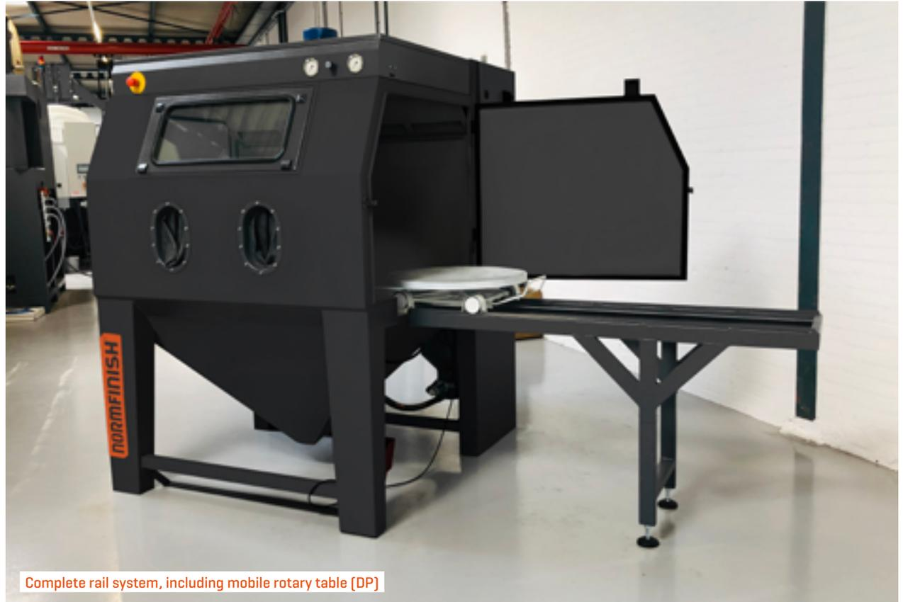
Complete rail system, including mobile rotary table [DP]
